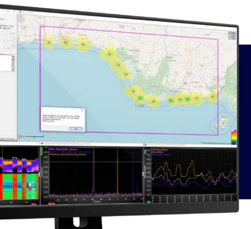
14 RFeye Arrays have been deployed on 15m tower (masts) based on geometry. The simulation shows RF Propagation Analysis with SOI running at 400 MHz with a power level of 44 dB at a roaming height of 10m. This can be changed.
