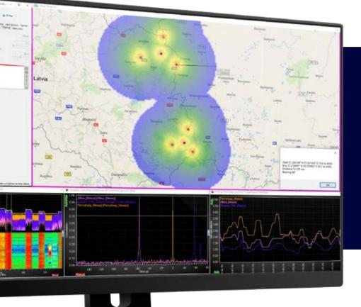
Eight RFeye Arrays are illustrated on 20m tower (masts) based on geometry. The simulation shows RF Propagation Analysis with a simulated signal running at 1.09 GHz at a roaming height of 1,000m. This can be changed.
